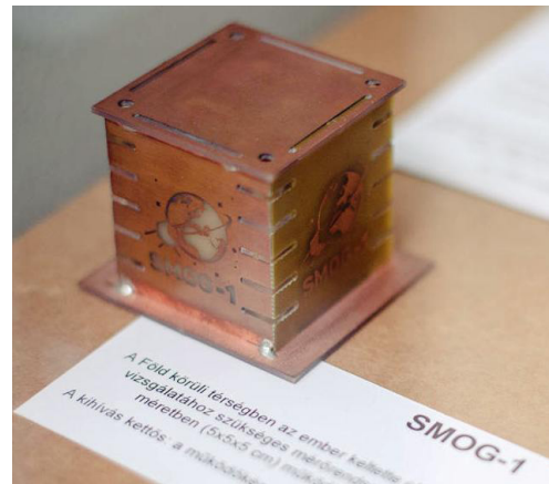
SMOG-1, the small satellite with the size of 1/8th of Masat
